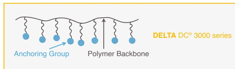
The compatibility of the dispersion control additive chain in various vehicles is determined by its chemical nature. Therefore different chemistries were developed by Delta Specialties, which are divided according to their chemical composition into two groups:
